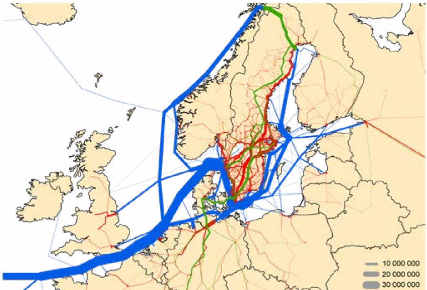
Figure 38. Total flows, in tonnes per month, using maritime shipping (blue), railways (red). (Source: Trafikanalys 2016).
