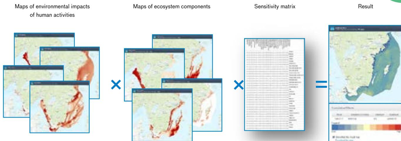
Figure 36. Method in Symphony, cumulative environmental impact. Symphony is the sum of all activities' impact on all nature values with different sensitivities. The calculation is made for every part of the sea, divided into a grid with quadrangles of 250 x 250 metres.
